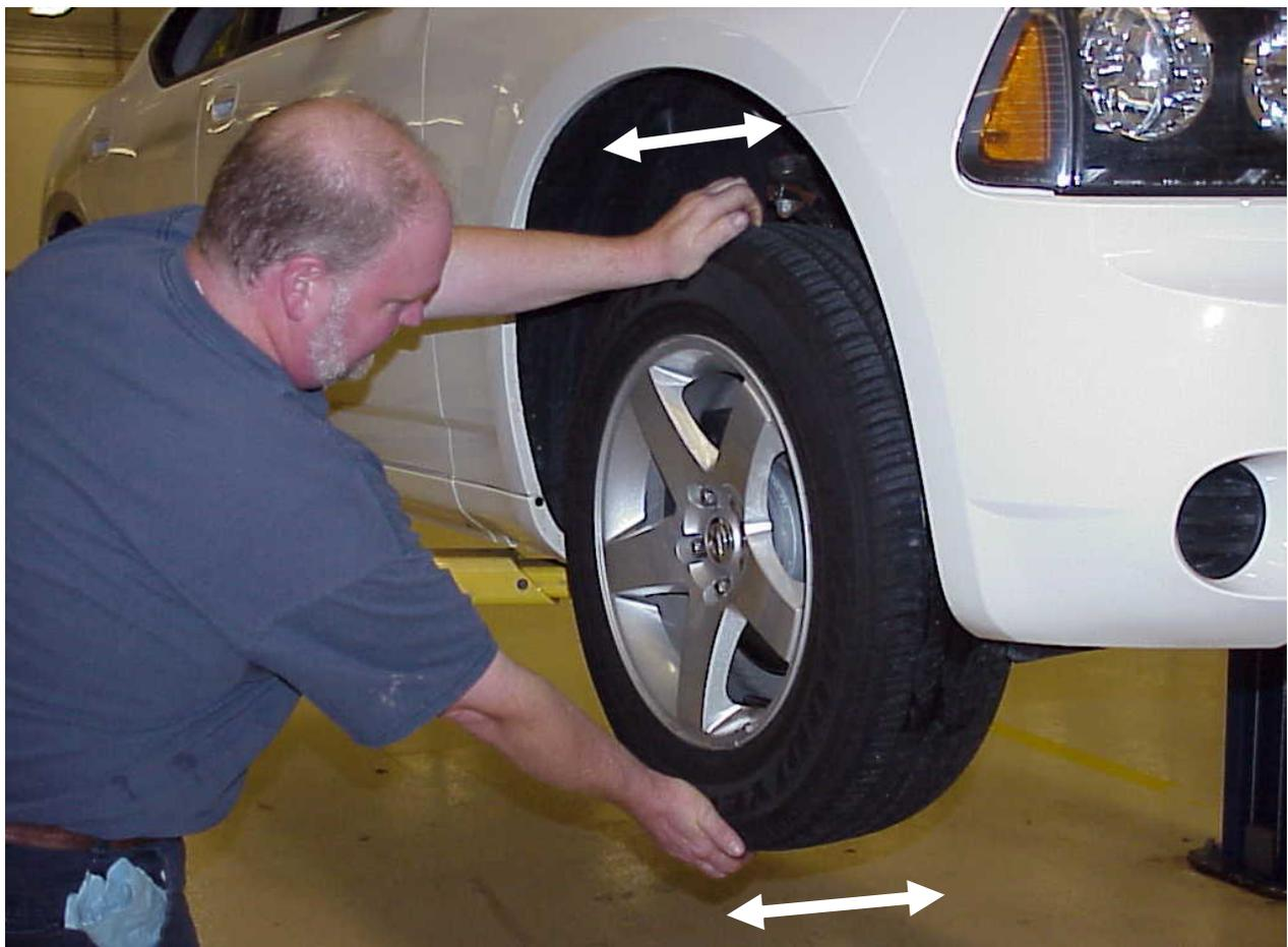
**Figure 1 – Check Front Wheels for Looseness**
