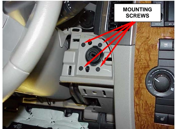
**Figure 8 - WIN Mounting Screws**
