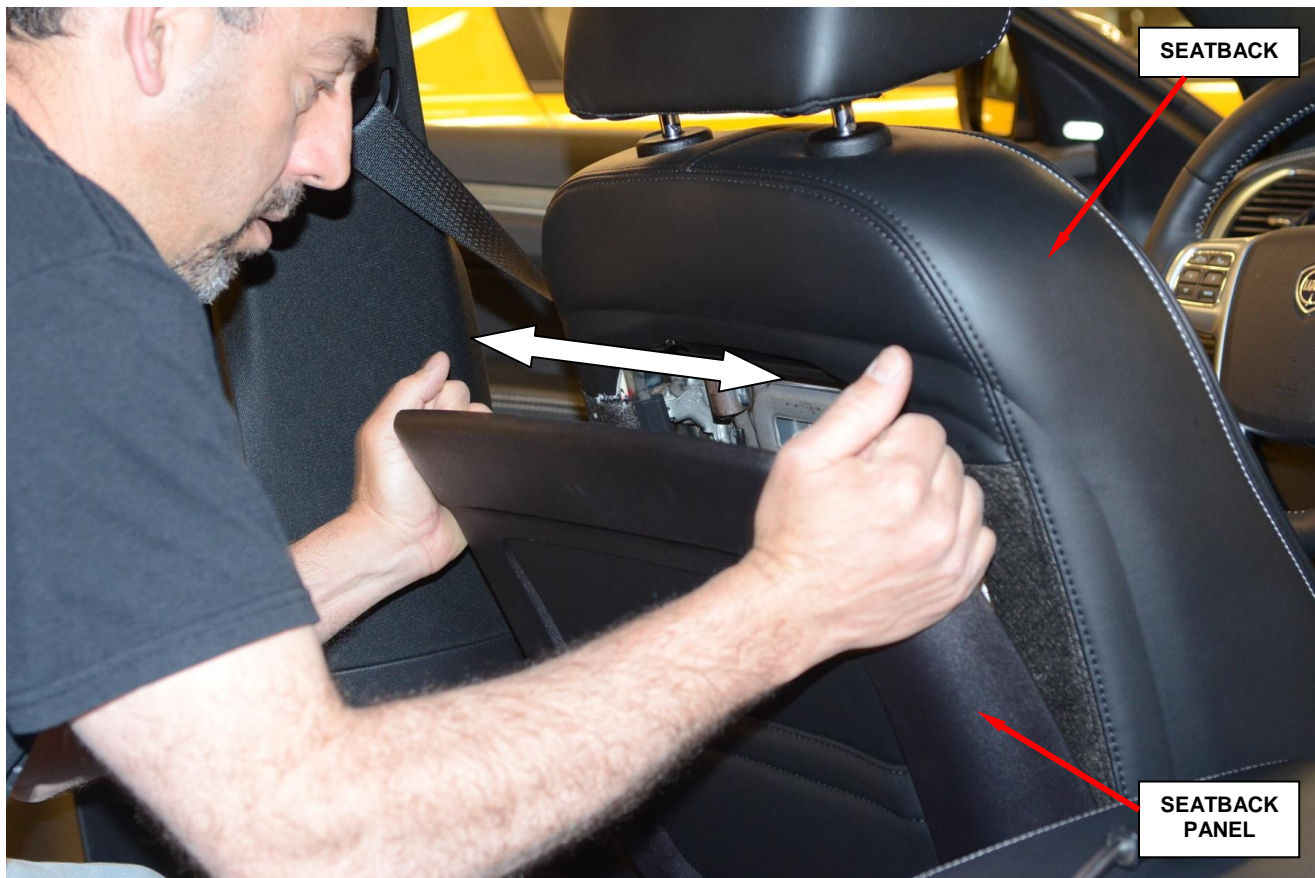
Figure 3 – Wiggle Seatback Panel Right and Left While Pulling Rearward
