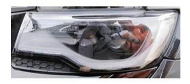
Fig. 1 Condensation Fogging Do Not Replace
