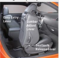
For easy access to the rear seat, pull upward on the easy entry lever, located on the passenger seatback; the seatback will dump forward and the seat will slide forward. You can also temporarily remove the seat belt from the guide loop on the seat and allow the seat belt to retract out of the way.
