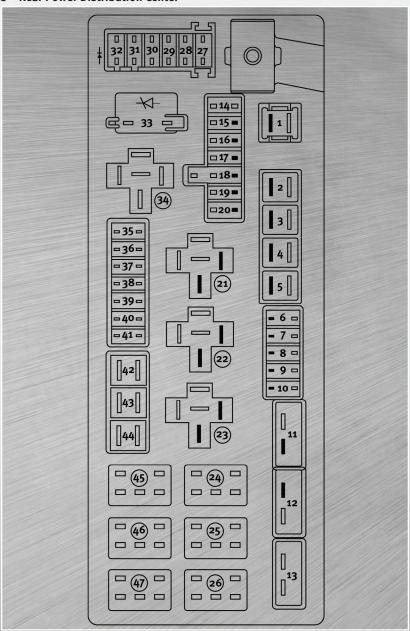
• There is also a power distribution center located in the trunk under the spare tire access panel. This center contains fuses and relays.
