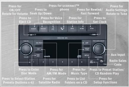
**NOTE:** uconnect<sup>™</sup> phone and Voice Recognition are vehicle options which must be ordered separately. The buttons on the radio will only be active if the vehicle has been equipped with the option.
